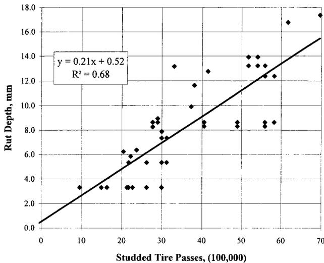
FIGURE 4 PCC studded tire wear rate results.
