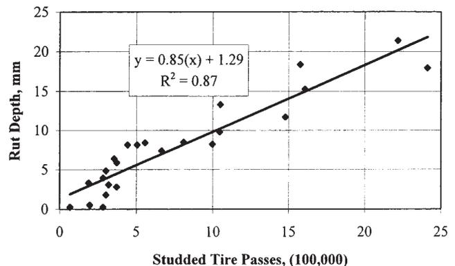
FIGURE 3 Asphalt studded tire wear rate results.
